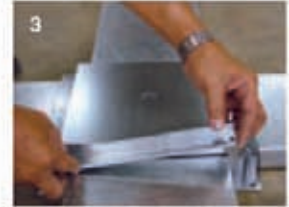
3 Align the trap frame bracket with the side blank plate
