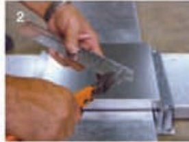
2 Cut off the pre-punched knockouts at the side blank plate
